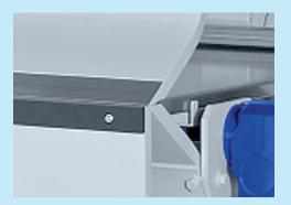
**Optimum clamping beam geometry**The special shape of the clamping beams enables a maximum bending angle of 145° while leaving a lot of free space inside the machine.
