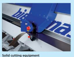
Manual or electric design with a cutting capacity of up to 1.5 mm (14 gg). Fitting it on the clamping beam eliminates constraining contours or force effects on the bending beam.
