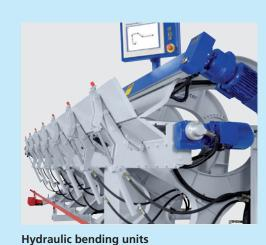
Each set of stand / tension arm is equipped with a hydraulically driven bending unit. Robust, sturdy construction for uniform bending forces along the full length.
